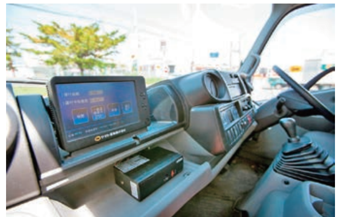
The See-T Navi system installed in a pickup and delivery vehicle
